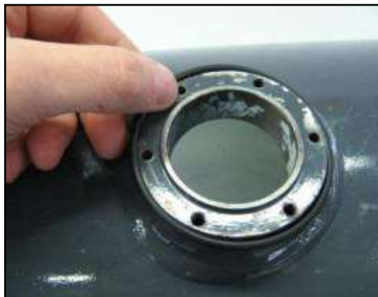
Figure 11: Placement of the O-ring gasket
