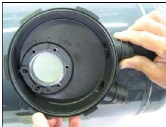
Figure 12: Positioning of the gas tight housing
