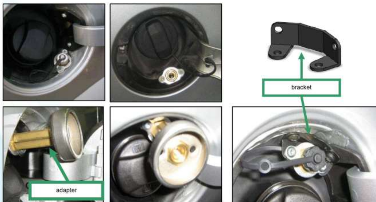
Figure 39: filling point installation
