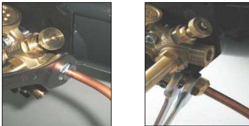
Figure 37: inlet and outlet fittings screwing 0° toroidal tank
