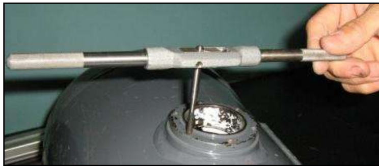
Figure 5: Removing of the paint from the screw threaded holes
