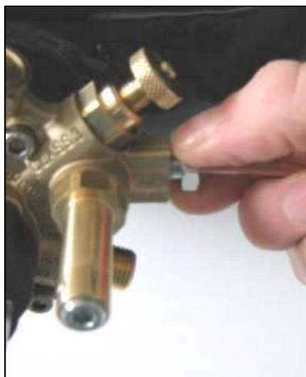
Figure 25: outlet fitting manual connection
